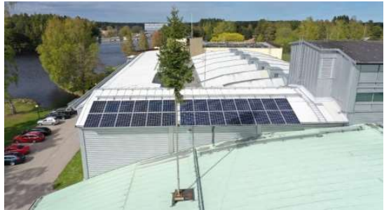
Figure 2: Experimental setup with simulated snow coverage (left) and for the tree shading experiment (right)
