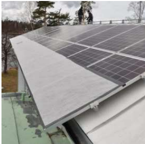
Figure 2: Experimental setup with simulated snow coverage (left) and for the tree shading experiment (right)
