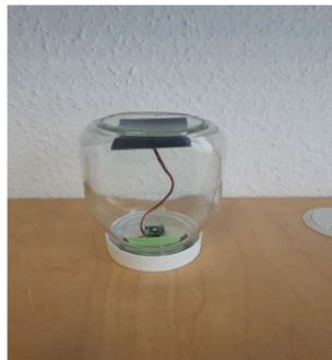
Picture 2: Assembled lamp; as housing a jam jar is used; a tilt switch (from mobile phone) allow switching by turning the lamp upside down.
